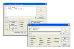
Queries can be used to easily solve all sorts of problems, such as entities colored by object and not on correct layers. In this example, all green objects that are not on the sanitary sewer layer can be located, their color changed to ByLayer and moved to the correct layer, all in one quick action.
