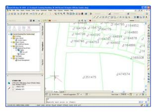
The Coordinate Tracking feature allows you to work within two different coordinate systems simultaneously. The AutoCAD X and Y coordinates in this example reflect the State Plane coordinates of the Current Drawing, and the UTM Zone 10 coordinates are displayed in the Coordinate Tracking box above. You can also enter coordinates into these fields, and click the digitize button, to precisely pick points in the alternate coordinate system.
