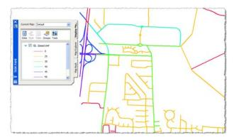
Thematic Mapping allows you to look at your data in new ways, without altering object properties. These streets were imported from an ESRI Shapefile to a single layer, colored by layer. Each street's speed limit was an attribute, converted to Object Data and mapped here by value using the Display Manager.
