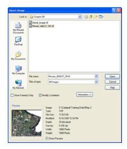
Map 3D offers a better way to insert aerial photographs and satellite imagery; it can read correlation data in all of the commonly available formats and use it to automatically insert the image at the precise location in your drawing.
