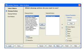
The Drawing Cleanup Wizard steps you through a variety of actions, offering many options to fine-tune each action to suit your needs. In interactive mode, each instance of a perceived error is marked with a symbol, allowing you to verify or ignore each correction, while the automatic mode fixes them all with one click.
