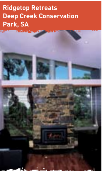
Passive solar design principles such as north facing glass in the living areas, roof overhangs and cross ventilation minimise the need for heating and cooling. These are supplemented by a slow combustion wood heater and ceiling fans for cooling.
