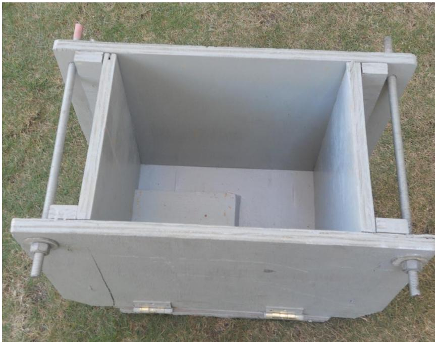
**Figura 8:** Caja o molde de plywood.
